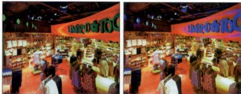
This Limited Too in Nashua, New Hampshire, uses an LED system with a changing color-wash effect on a colored sign. It creates the illusion of animation through the interaction of the colors.
